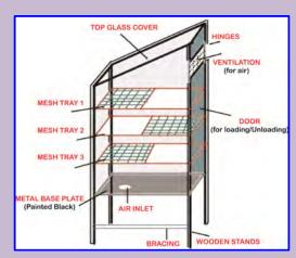
Schematic Layout of Mini Solar Dehydrator
