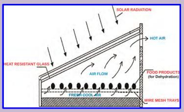
Dehydration Process in Mini Solar Dehydrator
