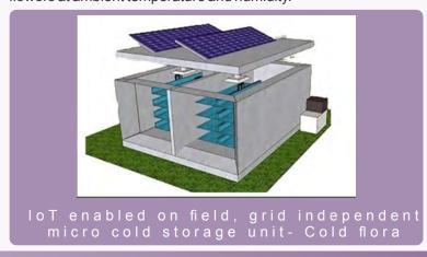
Clodflora has designed a renewable energy based wheel mountable, IoT-Enabled, on field/on market, grid independent micro cold storage unit 'ColdFlora' for storage as well as for transportation of floriculture produce that extends the shelf life and also preserve their freshness. The entire setup could be unloaded from wheels, and can doubly act as on field and on market storage.
