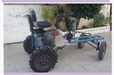
Small electric tractor after detaching the Reaper
